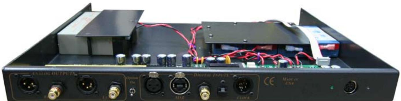
*Balanced digital* – The AES/EBU Professional input is the preferred input. The balanced nature of this input allows great cable lengths as well as total noise immunity.
