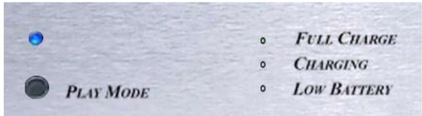
*FULL CHARGE LED* – This LED is lit when the charger is plugged in and the batteries are fully charged. This could take a day or two depending on temperature, line voltage and battery age.
