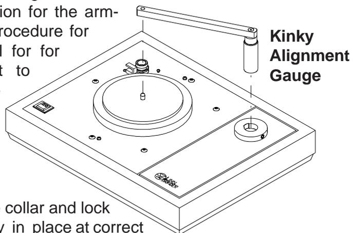
Fit the tonearm into the collar and lock the tonearm temporarily in place at correct height by lightly tightening the height locking screw in the tonearm base (See procedure on Mounting the Cartridge for details).
