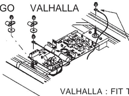
FIT THE SUB-CHASSIS EARTH TAG OVER THIS BOLT AND LOCK IT WITH A NUT.
