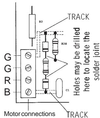
4. Trim the legs . The joints should be trimmed to about 2mm.
