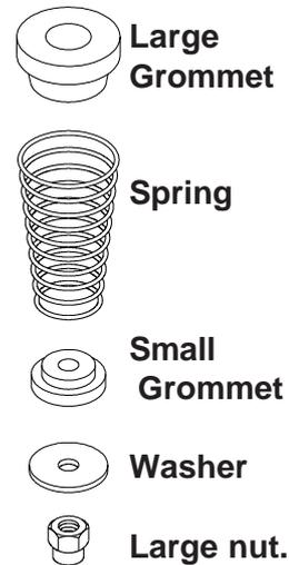
Each time you rotate a spring/grommet assembly, ensure that the entire assembly rotates during adjustment so that you do not introduce a twist in the spring. As you finish adjusting each spring, push up slightly and then release the washer on which the spring/grommet assembly rests. This will release any twist which may have been introduced into the spring.
