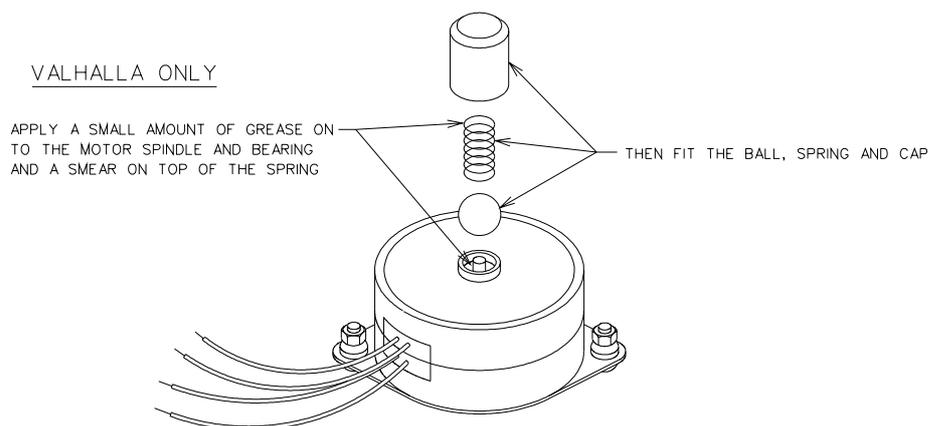
is properly greased. Use Linn black grease only. Refit the assembly to the bottom of the motor. After replacing the cap, push down on the motor pulley from above. The pulley should go down, then spring back to its original position when released. If you dislodge the cap when pressing down on the pulley, the spring assembly has not been properly seated in the cap, and/or there is grease on the mating surfaces of the cap and flange.
