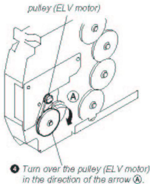
Remove the base (a not-supplied part shown at the bottom of page 114) installed in the CDM80, and rotate the PULLEY (GEAR) (1054 on page 114) clockwise to eject the disc.
