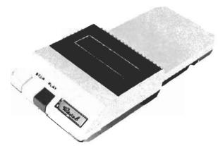
When there are two systems going in anything, there's always room for an adapter. This Japanese unit tackles the problem of playing cassettes on an eight track machine. It does it by playing the cassette and feeding the output to a magnetic head that mates with the playback head in the eight track machine.
