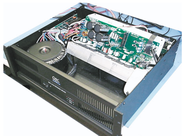
Figure 2. Prop the channel module assembly up on the chassis standoffs.
