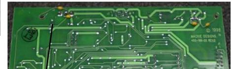
4. Add a 0.1uF capacitor across connector J2-pin 3 (+5VDC) and J2-pin 2 (digital ground).
