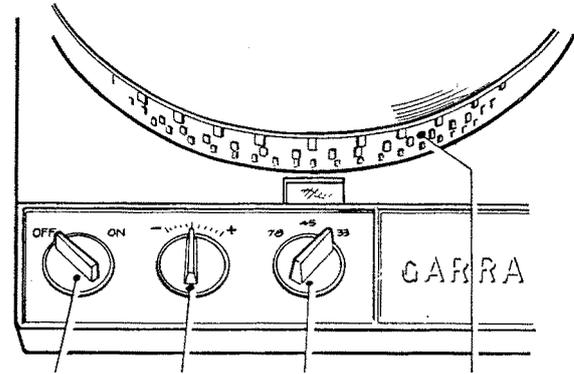
Motor Switch    Speed Adjuster    Speed Selector    Stroboscopic Markings
